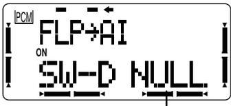
Switch direction display (NULL, UP, DOWN)
