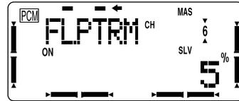
Note that the motion dictated by the Camber knob (CH. 6 flap trim knob) goes into both positive and negative camber from the neutral point, unless you set the F→A offset (see previous step). Also, note that if you don't set a small number or leave it inhibited (its default condition), you get HUGE motion of the trailing edge. You can set the approximate neutral point by matching the notch on the front of the knob with the slot in the knob holder.
