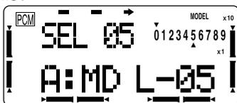
2. Press the right (>) CURSOR key twice to get to the model name function (NAME, p. 44). Use the CURSOR and DATA INPUT keys to spell out the name that you wish to appear on the screen, one letter at a time.
