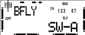
Shows that switch A turns the BFLY function on and off.
