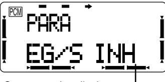
Current setting display (one of CH5, CH7, CH8 or INH). The default setting is INH (inhibited).
