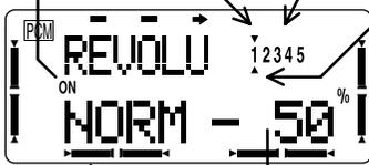
The bottom arrow shows the point on the five-point curve currently being set.
