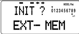
This warning appears when an [optional] **CAMPac** memory module is used in the transmitter for the first time. When the Plus (+) DATA INPUT key is pressed, initialization of the module begins, after which the memory module can be used. Once the module is initialized, the display will not appear again.
